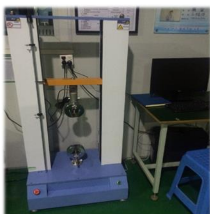
拉力测试&插拔测 (1000KG) Pull force/withdraw force
